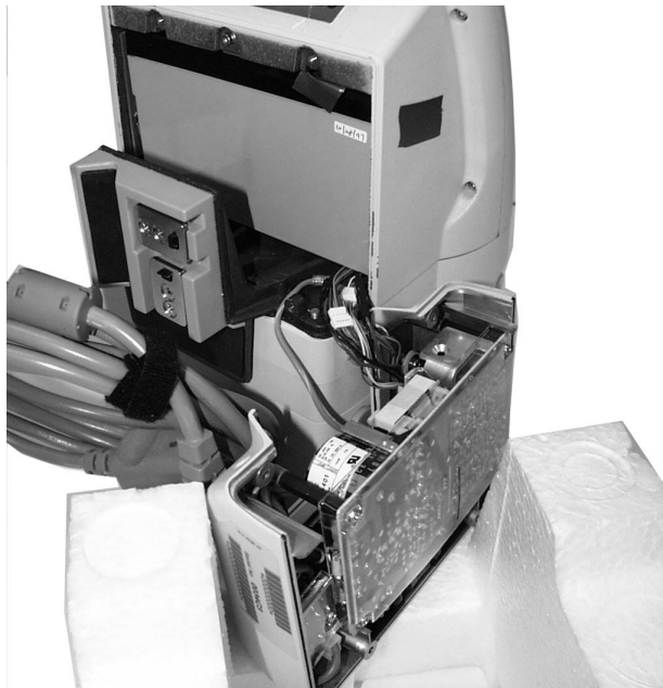
Figure 8-5 Supporting the Rear Housing of the Colleague 3 Pump during Disassembly
