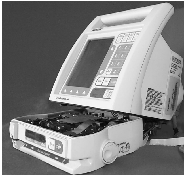
Figure 9-5 Supporting the UIM During AIL PCB Calibration
