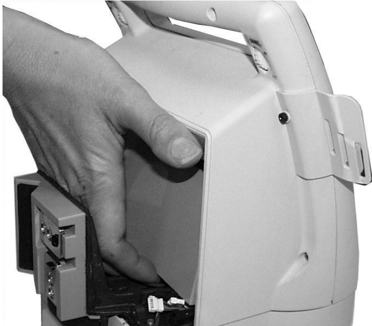
Figure 8-6 Removing the Rear Battery Using Your Hand
