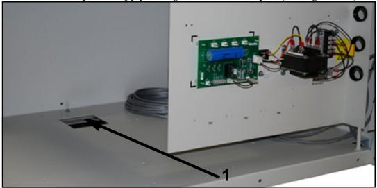
**17** Feed the PBL cable (supplied with the collimator) from the collimator power supply through the cable access port (1 in Figure 2-11).
