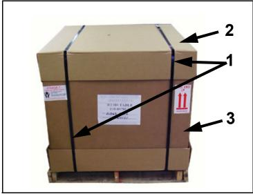
Figure 2-2. Steel Shipping Straps
