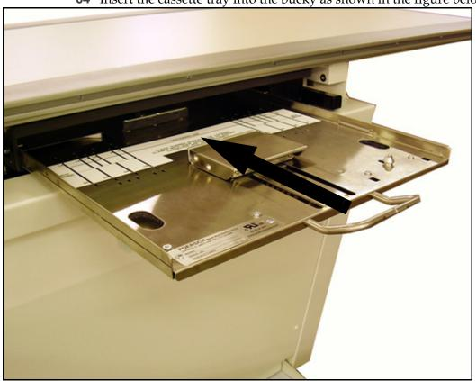
**64** Insert the cassette tray into the bucky as shown in the figure below.
