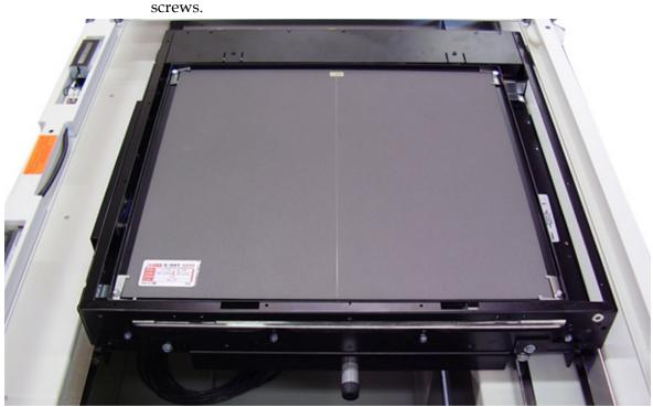
**40** Install the grid as shown below and secure it in place with clamps and screws.
