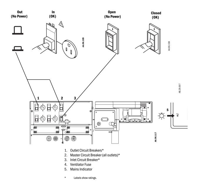
Figure 5-1 • Circuit breakers, fuse, and the mains indicator
