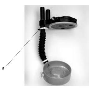
Note: Optionally, the bypass assembly can be divided into two smaller sections for easier cleaning by releasing the top clamp (a) and pulling the hose from the assembly. When reassembling, reattach the hose to the bottom part of the assembly. Secure the hose with the clamp and pinch the clamp one notch past finger-tight with pliers.
