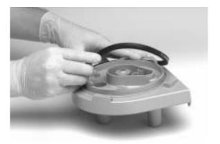
Do these steps in the opposite order to assemble the bellows. If you see a dust-like powder on the housing or the bellows, apply a thin layer of KRYTOX lubricant to the ribs of the bellows housing. Make sure the lubricant is applied smoothly and there are no lumps.
