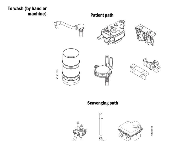
Use a mild detergent (pH <10.5). Then, rinse and dry completely. All parts except the  $O_2$  sensor, and flow sensors can be washed.
