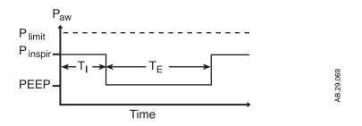
Figure 7-3 • Pressure control diagram
