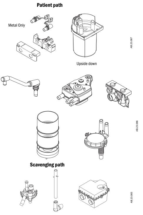
Autoclave at  $134^\circ\text{C}.$  Inspect the parts for deterioration. The User Maintenance section tells you how to do this.
