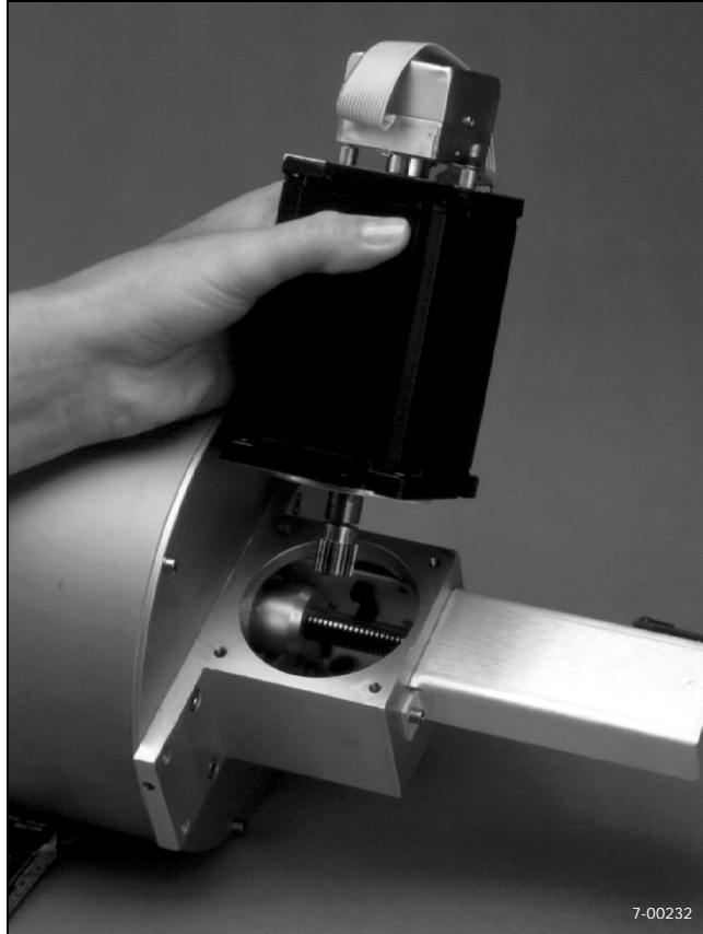
Figure 8-48. Gear mesh procedure: Positioning motor encoder
