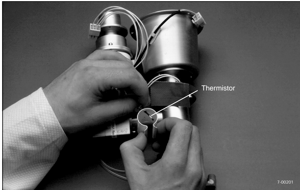
Figure 8-37. Threading thermistor through flow sensor heater clip
