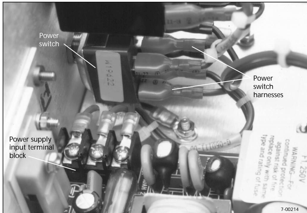
Figure 8-55. Power supply input terminal connections
