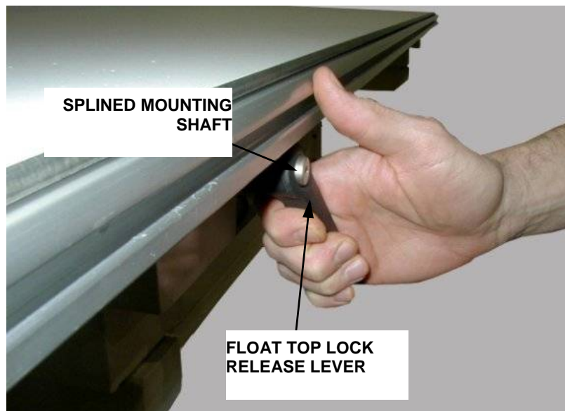
Figure 6. Float Top Lock Release Lever (Engaged Position)
