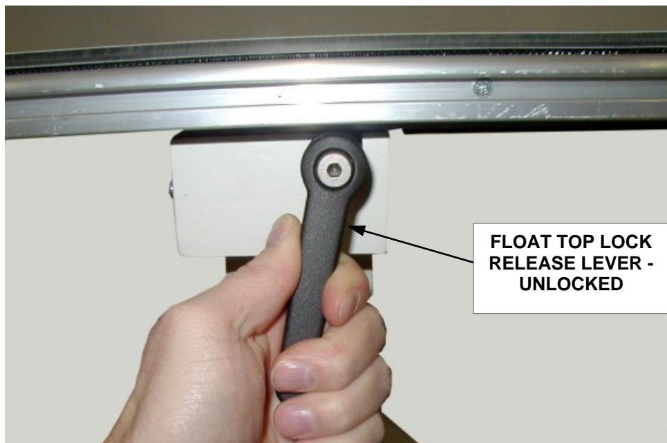
Figure 10. Float Top Lock Release Handle in Un-Locked Position
