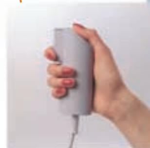
The hand-held fluoro switch controls release of exposure and image storage on the fly
