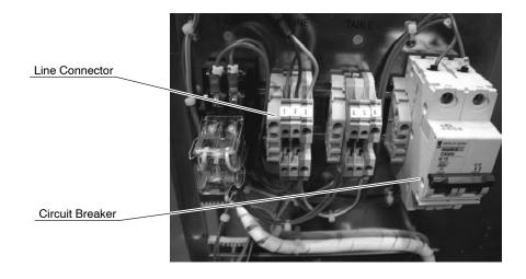
c. Turn On the Circuit Breaker. Visually check that all green lights and LED DS1 are lit on the Charger Board.
