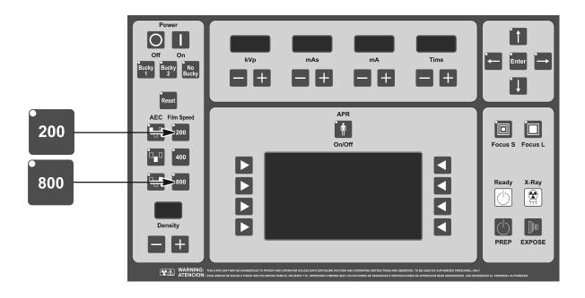
3. Enter Auto-calibration mode by pressing the "Power On" and "kV increase" push-buttons simultaneously for 2 seconds. After releasing both push-buttons, code "222" will be flashing on the Console waiting for confirmation to then enter Auto-calibration mode.
