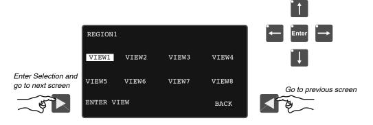
5. **Modify the View name**. Press "Enter" to edit the name of the selected View. The first letter of the name is highlighted, the "Up/Down Edit-Arrow" buttons will change the letter in alphanumerical order (plus underscore and blank), the "Right/Left Edit-Arrow" buttons will scroll in the word. Once the name is written, press "Enter" to save the new View name. If necessary, repeat this process to rename other Views.
