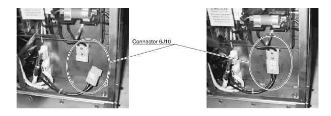
Connect the Line Power cable to Line Connector (wire-1 to left, wire-2 to middle, ground wire to right). These connections are color coded.
