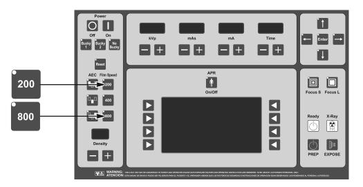
2. Press the "mA Increase" push-button until you reach the maximum mA capacity. Press the "mA Increase" push-button twice more to reach the Extended Memory Code "E02", that will appear on the mA Display.
