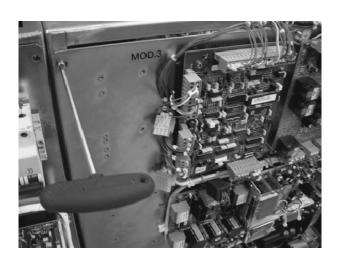
6. The Terminal Strip 4TS2 is located on Module 4 (back of Module 3) of the hinged door. Connect the X-ray Tube Rotor wiring as follows:
