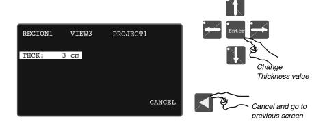
After pressing "Enter", the Console automatically displays all the radiographic parameters (kVp, mA, mAs, Time), selections (Workstation and AEC) and SID indication related to that Region/View/Projection.
