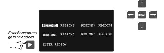
3. <u>Modify the Region name</u>. Press "Enter" to edit the name of the selected Region. The first letter of the name is highlighted, the "Up/Down Edit-Arrow" buttons will change the letter in alphanumerical order (plus underscore and blank), the "Right/Left Edit-Arrow" buttons will scroll in the word. Once the name is written, press "Enter" to save the new Region name. If necessary, repeat this process to rename other Regions.
