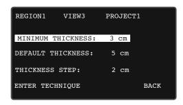
Modify the Radiographic Technique Values. In order to modify the Radiographic Technique values for a specific Region/View/Projection, press the Display Selector close to "ENTER TECHNIQUE".
